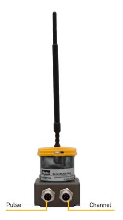
Pulse: High-to-low voltage pulse transition from external device
