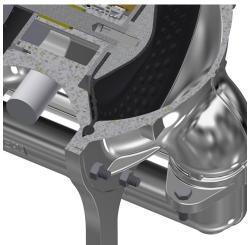
All DEPA® SteriTec™ pumps are equipped with our Closed Surface Diaphragms (CSD). The CSD has an extended life time and eliminates leaks, due to an integrated insert, which eliminates a potential leak path in the pump. The pump maintenance is simplified and requires only hand tightening of the diaphragm. Its modular design ensures all diaphragms are interchangeable with all DEPA® pumps, and its clean surface reduces the build-up of impurities, improves flow and increases energy savings.
