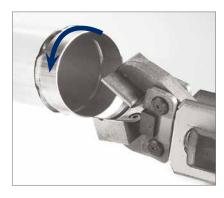
3. Re-open the jaw to remove the pipe. Position the end of the jaw next to the lug mark: this will help to prevent overlapping the lugs.
