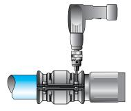
6. Using a drill, fully tighten the clamshell bolts in a cross pattern
