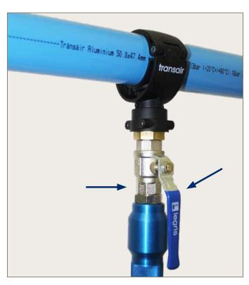
2. Thread the drilling tool onto the ball valve. Ensure the valve is open then fully drill the hole.
