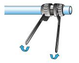
6. Complete the assembly by tightening the connector one-half (1/2) turn with the Transair spanner wrenches
