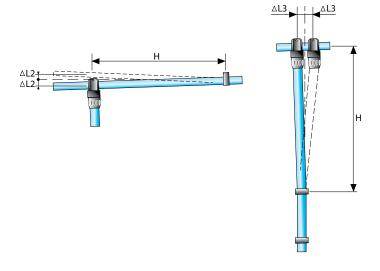
The length variation  $\Delta L$ , calculated for the Transair® line, must always be equal to or less than  $\Delta L2$  and  $\Delta L3$ . If this is not the case, then an expansion loop, using Transair® flexible hose, must be added.
