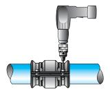
6. Using a drill, fully tighten the clamshell bolts in a cross pattern Torque Specs: 7.38 lb-ft to 29.5 lb-ft
