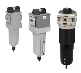
Note: To optimize the life of coalescing element, it is advisable to install a pre-filter with a 5 micron element upstream of the coalescing filter. To optimize the life of an Adsorber, if used, it is advisable to install a Coalescing Filter upstream of the Adsorber. Adsorber element should be replaced approximately every 1000 hours of service.
